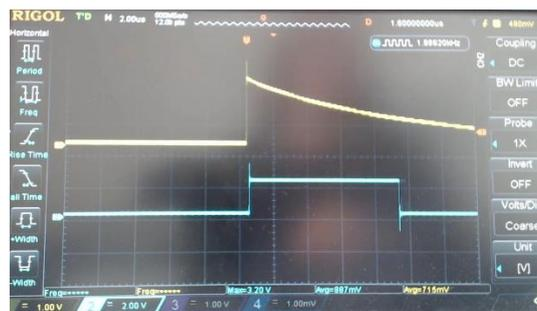
The yellow line comes directly from the CAEN DT4800 signal generator while the blue one is drawn by the *LEMO Output* of the SciDK Development Board programmed with SciCompiler and represents the interval in which the first signal has a value greater than the programmed **Fixed Threshold** of 3000.
